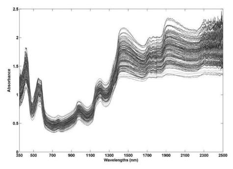
Fig. 1. Spectra collected from intact pork loins using a fiber-optic NIRS instrument from LabSpec®Pro.
