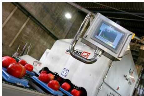
Fig. 2. Arils extraction technology: A patented principle of operation (i) Current Field Capacity: up to 56 fruits per minute; (ii) Operates in 10 countries with over 30 installations.
