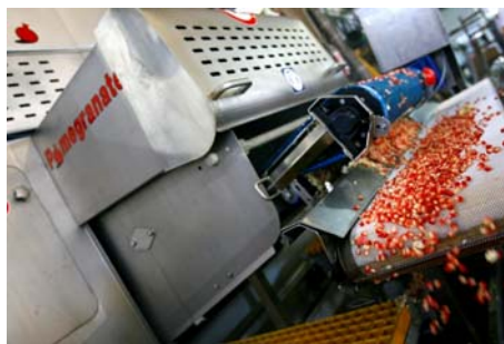
Fig. 2. Arils extraction technology: A patented principle of operation (i) Current Field Capacity: up to 56 fruits per minute; (ii) Operates in 10 countries with over 30 installations.
