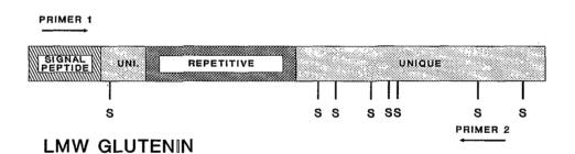
Fig. 5. Diagram of a LMW glutenin gene. Arrows indicate the position of primers used for PCR analysis. S indicate the position of codons coding for cysteine residues.
