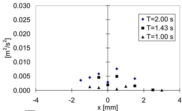
a)  $\overline{u^2}$  at cross section 5 mm from the nozzle.
