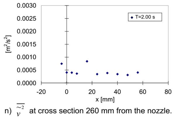
Fig. 3. Cross-sectional profiles of  $\overline{\tilde{u}^2}$  and  $\overline{\tilde{v}^2}$ .
