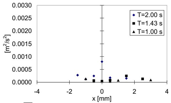
b)  $\overline{v^2}$  at cross section 5 mm from the nozzle.
