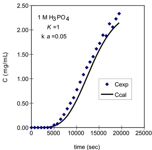
Figure 3. Breakthrough and fitting curve of uranium in 1 M  $H_3PO_4$ .
