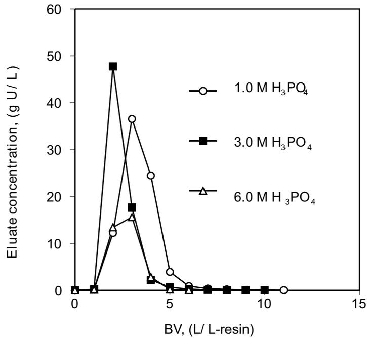
Figure 6. Elution curves of uranium in 1, 3 and 6 M H<sub>3</sub>PO<sub>4</sub>.
