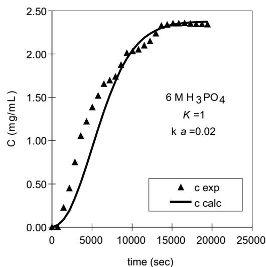
Figure 5. Breakthrough and fitting curve of uranium in 6 M  $H_3PO_4$ .
