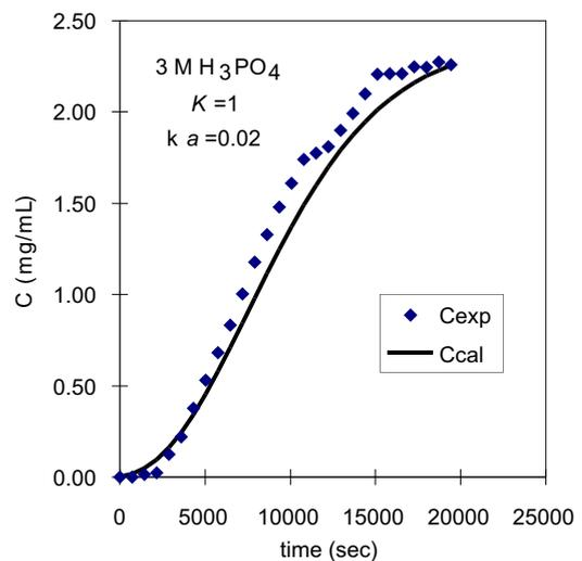
Figure 4. Breakthrough and fitting curve of uranium in 3 M  $H_3PO_4$ .
