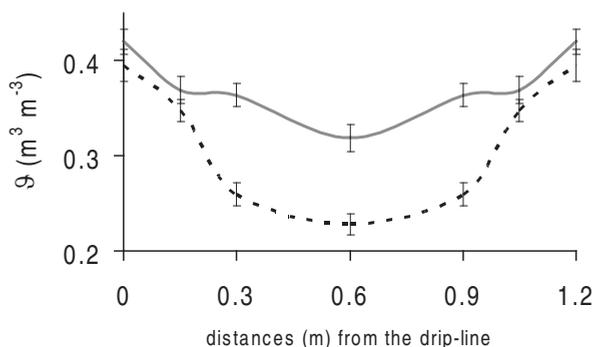
**Figure 2. Volumetric moisture (at -0.3m depth) measured during the tomato season in the transect between two contiguous drip-lines under two water regimes: full irrigation (solid line) and stress (dashed line).**
