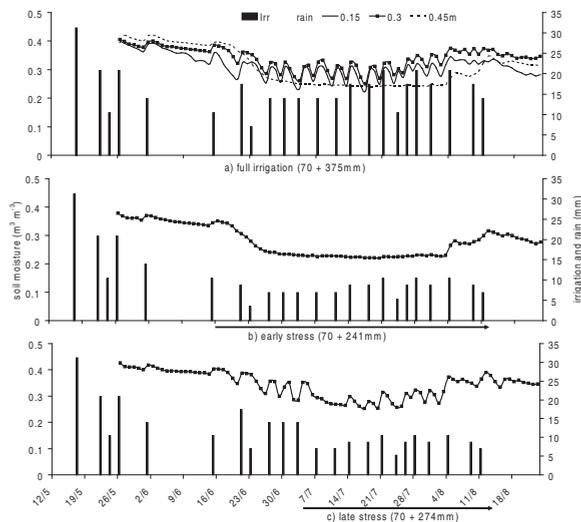
**Figure 1.** Soil moisture measured by the TDR technique at -0.15, -0.30 and -0.45m in a), and at -0.30m in b) and c). Amounts of irrigation (solid) and rain (dashed) are represented by vertical lines. Arrows in b) and c) indicate the temporary stress periods.
