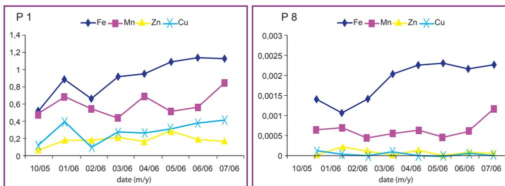
**Fig. 7 & 8: spatial and temporal variations of MTE elements in surface water at points 1 and 8 (Fe, Mn, Zn, Cu)**
