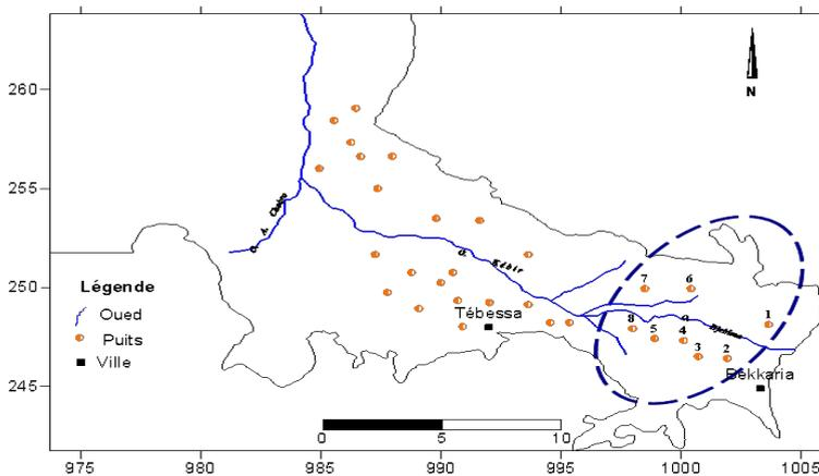
**Figure 9: distribution of the sampled water wells.**
