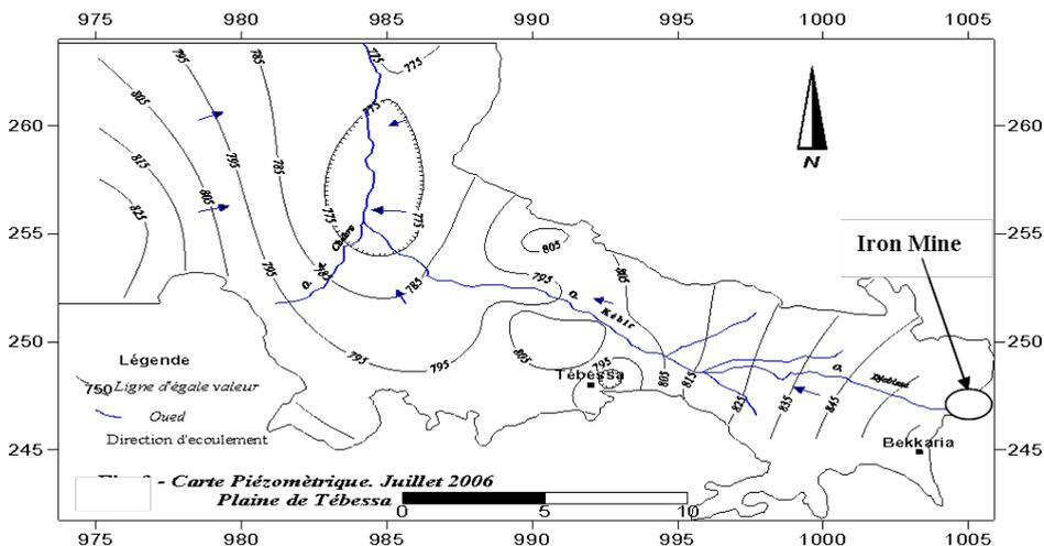
**Figure 2: Piezometric map of the shallow aquifer (July 2006).**
