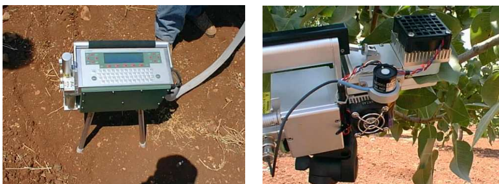
Fig. 3 Portable photosynthetic system LICOR 6400 for measuring leaf gas-exchange: system console and leaf chamber with a tree leaf clamped into.
