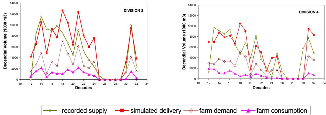
Fig. 6. Comparing the 10-day recorded supply with the SEDAM simulated delivery farm water use and consumption for Division 2 and 4 of HID.
