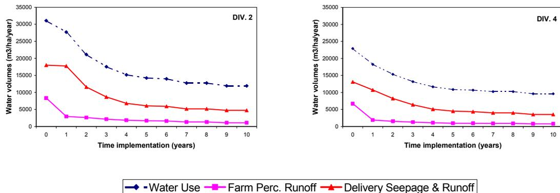
Fig. 11. Foreseen time evolution of the total water use, seepage and branch canals runoff, and farm percolation and runoff for Division 2 and 4.
