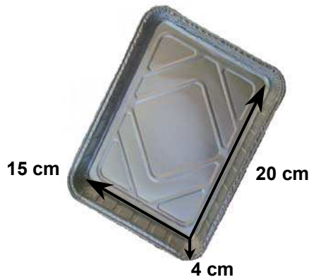
Figure 2. Aluminium container dimensions used in the experiment
