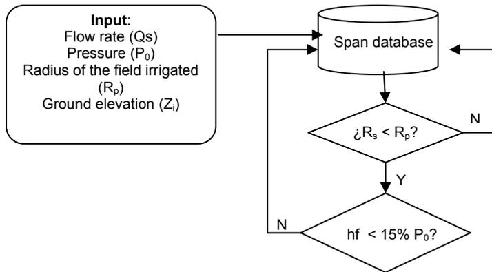
Fig. 2. Schematic representation of hydraulic simulation model.
