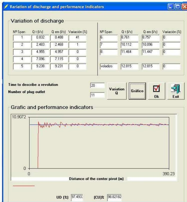
Fig. 5. Window showing results on discharge variation for each span and along the lateral, including the DU and CU indicators of uniformity.
