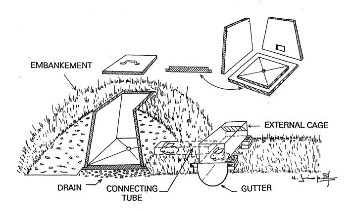
Fig. 1 - First prototype of the underground cell housing.
