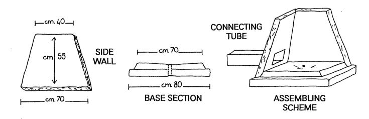
Fig. 2 - Draft of the cement underground cell.
